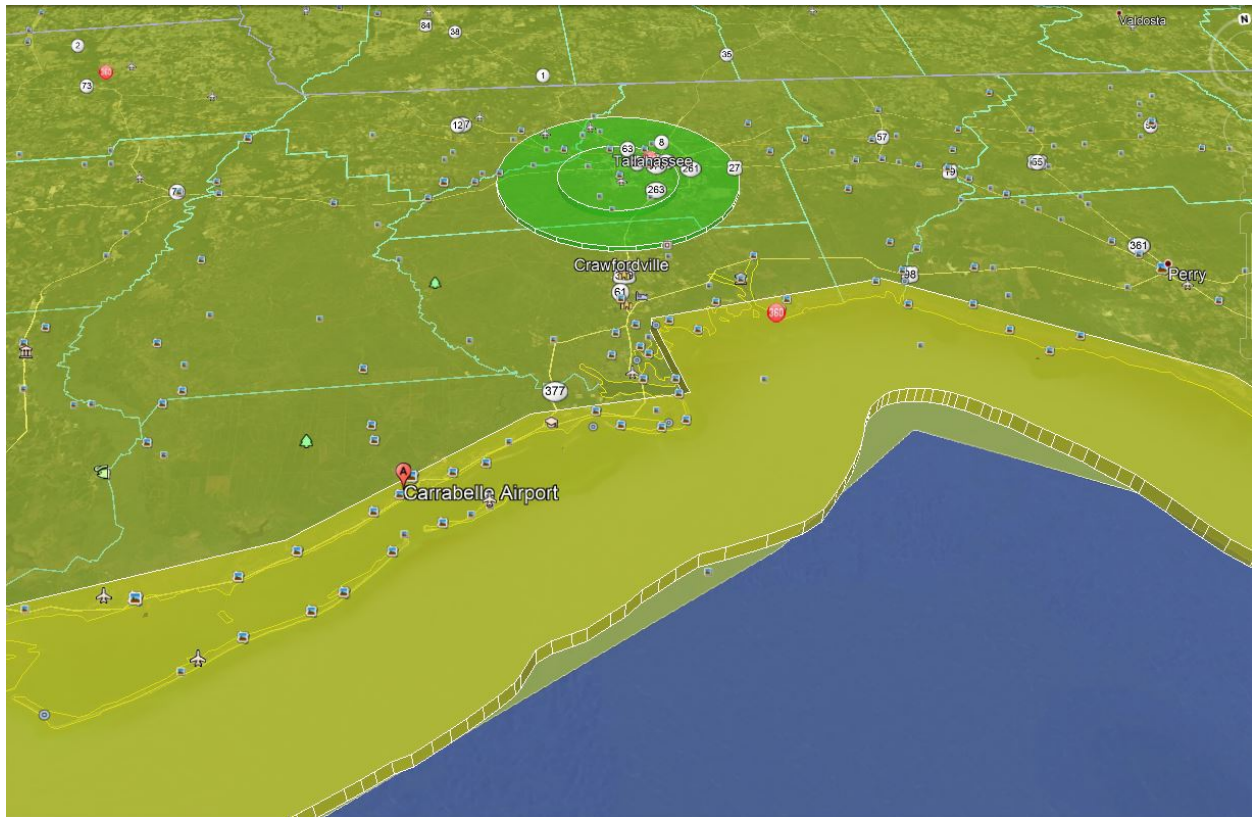
Figure 2.31. Airspace Classifications around Carrabelle Airport. Class E Space is yellow and Class C space is green; Class G airspace is not depicted on aeronautical charts
